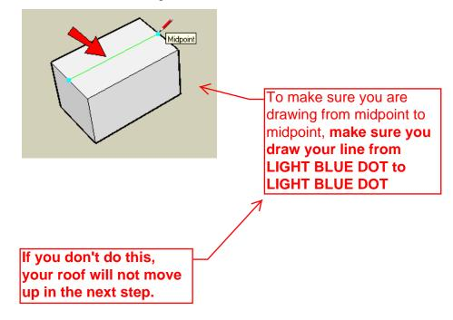
3. Use Move on this line, pulling it up (in the blue direction) to make the roof.
