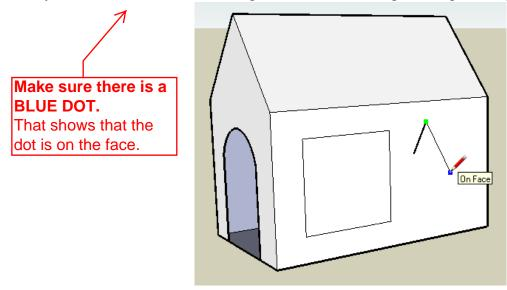
10. Be sure to end the window shape where you started. If your lines are correct, the edges around the window will be thin.
